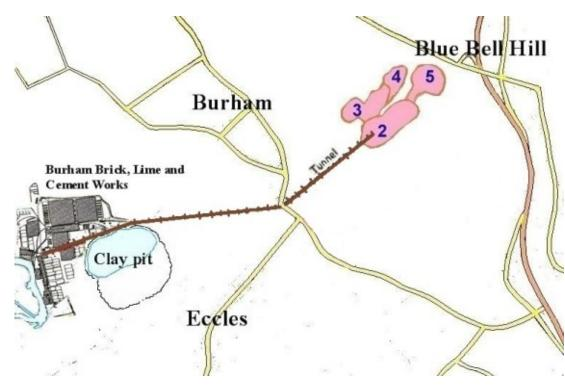
The first action was to construct a line from the works to sections number 2-3, including an 800m tunnel. This allowed easy transport of Chalk from the Upper Culand pit, especially sections 2, 3 and 4. The photo of the tunnel was taken just to the NE of Petts Farm. Today, the entrance in section 2 is gridded over to allow bats in and out, but to keep humans out.
